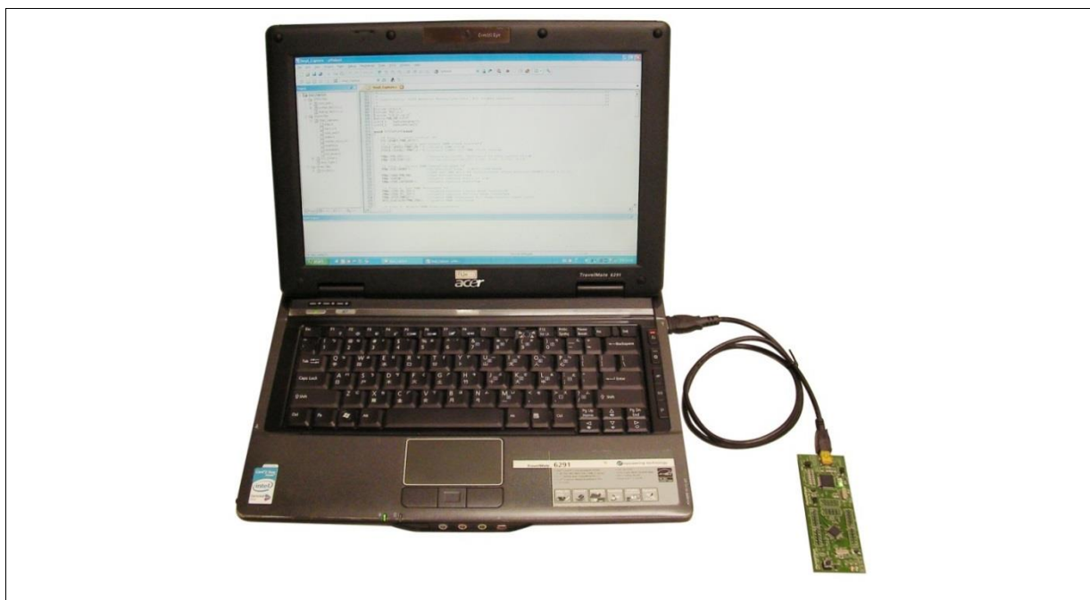
Figure 4-1 NuTiny-SDK-M0519 Hardware Setup
